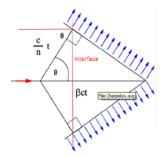
We have constructive interference when  $\cos\theta = vT/(v_sT) = v/v_s$ .
