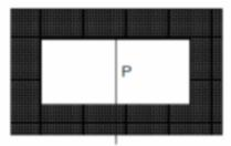
Gas at standard temperature and pressure is initially in the left-hand compartment of the device shown above. The right-hand compartment is initially evacuated. The volumes of the two compartments are the same, and the entire device is thermally insulated from its surroundings. If the partition P separating the two compartments is rapidly pulled out sideways, which of the following will be true?
