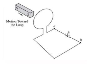
The bar magnet shown in the figure above is moved completely through the loop. Which of the following is a true statement about the direction of the current flow between the two points a and b in the circuit?
