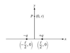
A pair of electric charges of equal magnitude q and opposite sign are separated by a distance  $\ell$ , as shown in the figure above. Which of the following gives the approximate magnitude and direction of the electric field set up by the two charges at a point P on the y-axis, which is located a distance  $r >> \ell$  from the x-axis?
