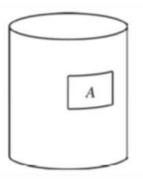
Consider the closed cylindrical Gaussian surface. Suppose that the net charge enclosed within this surface is  $+1 \times 10^{-9}$  C and the electric flux out through the portion of the surface marked A is  $-100 \text{ N} \cdot \text{m}^2/\text{C}$ . The flux through the rest of the surface is most nearly given by which of the following?
