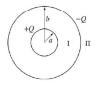
Two thin, concentric, spherical conducting shells are arranged as shown in the figure. The inner shell has radius a, charge +Q, and is at zero electric potential. The outer shell has radius b and charge -Q. If r is the radial distance from the center of the spheres, what is the electric potential in region I (a < r < b) and in region II (r > b)?
