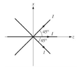
Three long, straight wires in the xz-plane, each carrying current I, cross at the origin of coordinates, as shown in the figure above. Let  $\hat{\mathbf{x}}$ ,  $\hat{\mathbf{y}}$ , and  $\hat{\mathbf{z}}$  denote the unit vectors in the x-, y-, and z-directions, respectively. The magnetic field  $\mathbf{B}$  as a function of x, with y = 0 and z = 0, is
