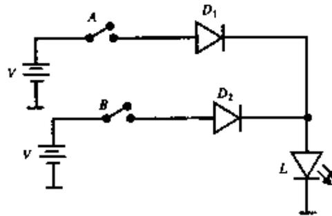
Fig. 7.4 Positive-logic OR gate using diodes.
