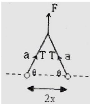
The vertical force on each particle is  $T \sin \theta$ ,  $2T \sin \theta = F$ .The horizontal force on each particle is  $T \cos \theta = F \cos \theta / (2 \sin \theta) = F / (2 \tan \theta)$ .
